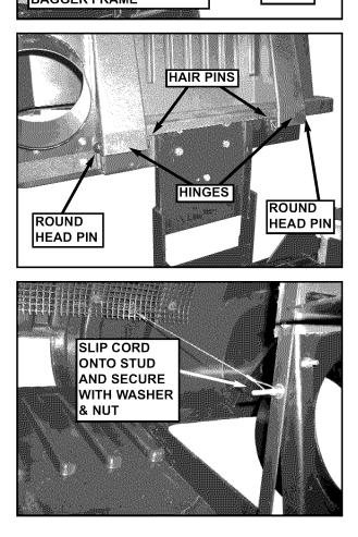
**STEP 13:** Hook bottom of bagger frame onto pins in bottom of bumper mount plate. Then slide locking rod through aligned holes in bagger frame and bumper mount plate, securing with bridge pin.
